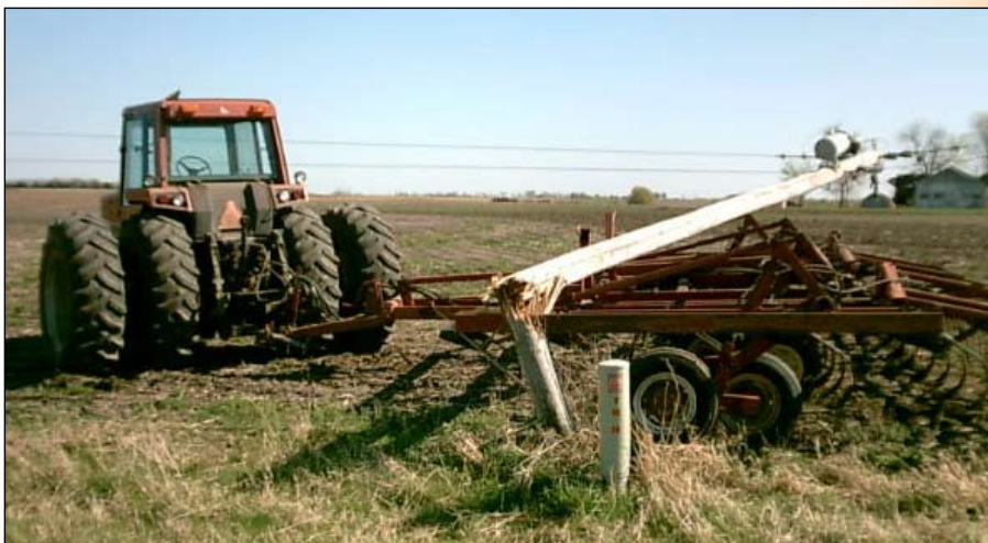
A primary line carrying 7,200 volts of electricity fell on this tractor when the driver came too close to the electrical pole in northeast Kansas.
